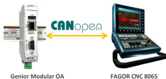
1) Schematic illustration of the CANDTA connection between Genior Modular OA and FAGOR CNC 8065
